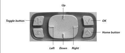
The cursor can also be used to navigate through devices and pages on Pronto NG's touch screen.
